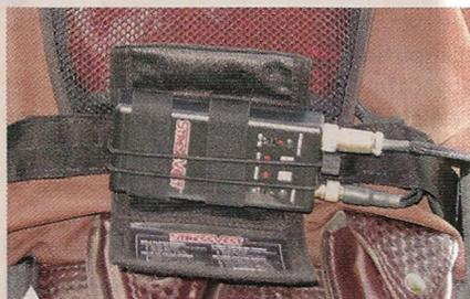
The rear-worn controller for the StressVest has four modes and 12 different settings.
